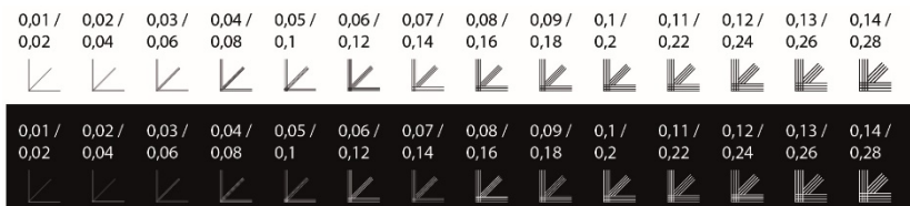
Fig. 1. The part of the control wedge for 0,01–0,15 mm width positive and negative micro-lines arranged individually
