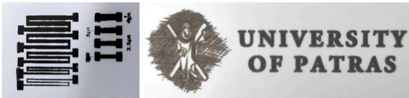
Figure 4. Representative screen printed patterns using the G/MWNT-f-OH hybrid with total solids carbon/resin ratio 55/45 printed on (left) smart-paper type-2 and (right) extra premium photo paper
