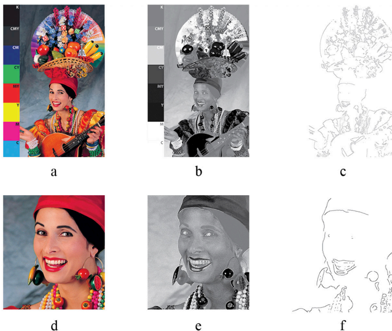
Fig. 3. A test image with the security mark; a – composite image; b – yellow channel; c – fluorescent channel; d, e, f – magnified fragment of the image.
