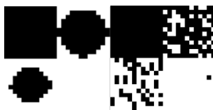
Fig 2. Raster dots with 0%, 20%, 50% and 100% dot area rate after printing model: left — regular, right — irregular
