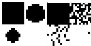
Fig 1. Raster dots with 0%, 20%, 50% and 100% dot area rate: left — regular, right — irregular
