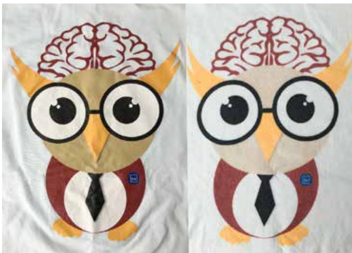
Fig 6. Thermal transfer printing (the first) and direct printing (second) temperature 60 °C
