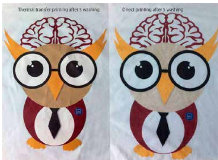
Fig 5. Thermal transfer printing (the first) and direct printing (second) 30 °C
